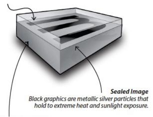
Aluminum Layer The rigid aluminum base will not peel, crack or delaminate.
